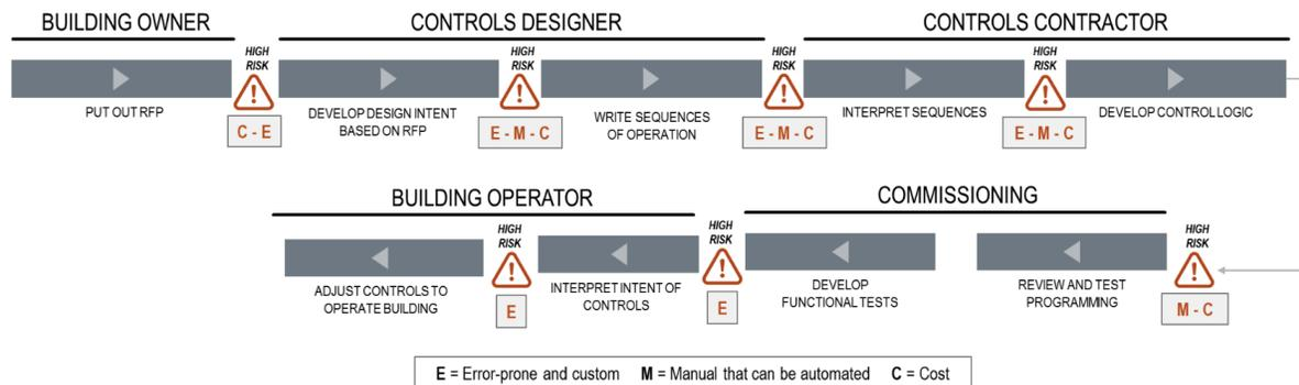
Figure 1: Conventional control delivery workflow (Paliaga et al., 2020)
