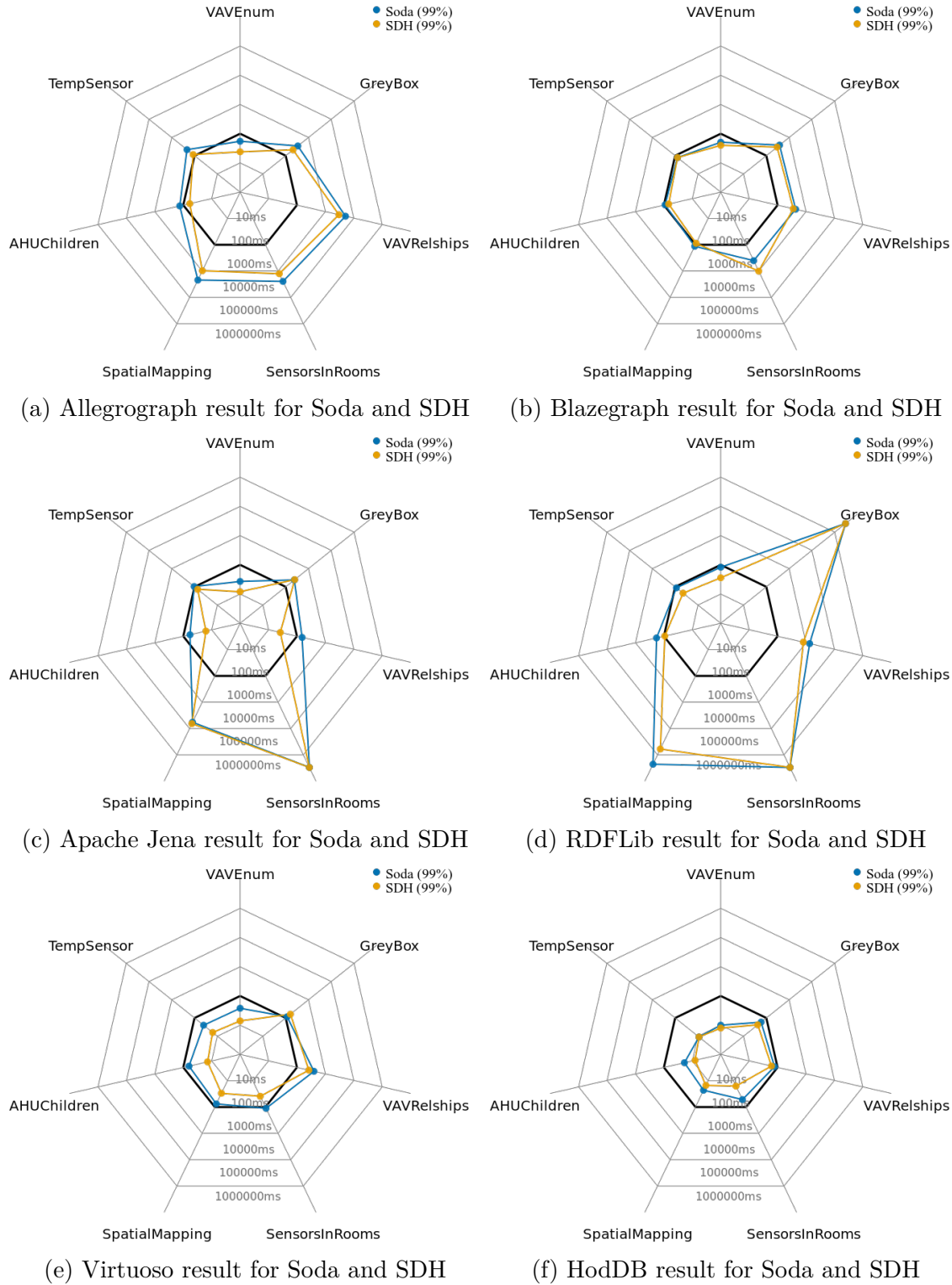
Figure 7.3: Radar plots showing the 99th percentile latency for each of the benchmark queries over the two larger buildings. All times are in milliseconds. The bold line represents the 100ms target. Note the log scale.
